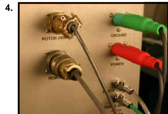
Connect the power, ground, motor, gas and remote (if applicable) of the welding head to the power supply.
