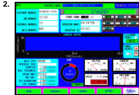
Push the CALIBRATE button then select the proper switch setting on the Rotor Driver then push CALIBRATE.
