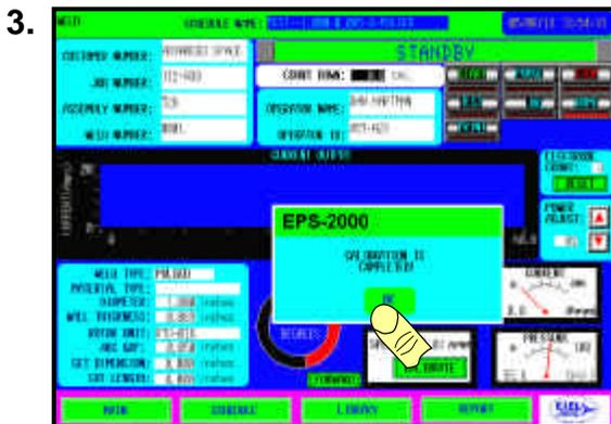
During calibration 4 revolutions will be made and timed. When calibration is complete, push OK.
