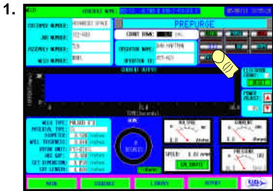
After Rotor Driver calibration a test weld can be made to be certain of proper settings and calibration by pushing TEST.
