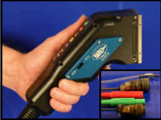
A welding head is required to operate the EPS-2000 Power Supply. Above is the Exel RDR-05 Rotor Driver.
