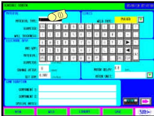
Enter the Material Type that will be welded by touching the field and using the QWRTY keypad that appears.
