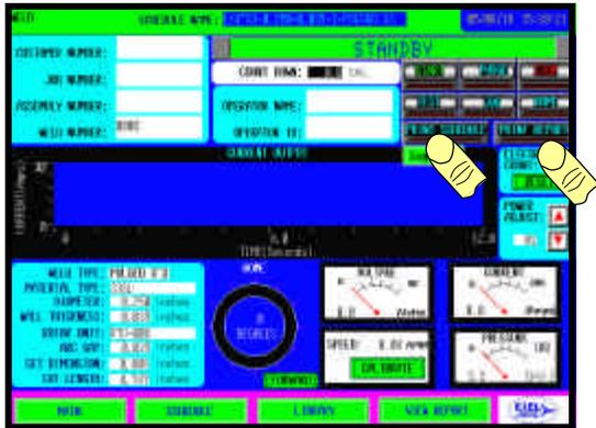
To print from the power supply, select either PRINT SCHEDULE or PRINT REPORT the onboard printer will print the desired form.
