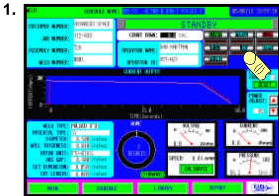
Push the JOG button to rotate the weld head. The head will rotate only when the button is pushed.
