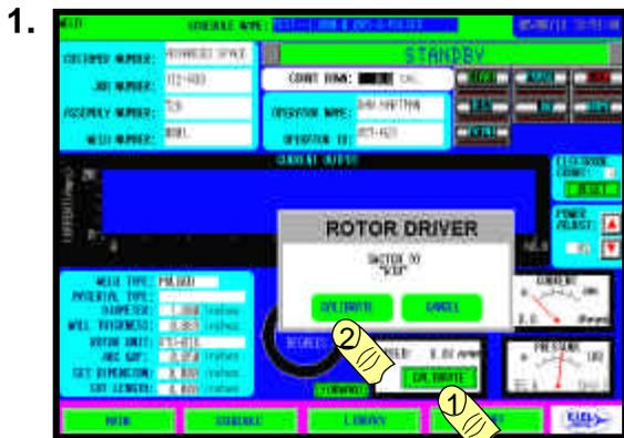
When loading a new weld schedule or turning power on, the Rotor Driver or motor must first be calibrated.
