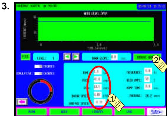
Enter Level 1 data and click UPDATE GRAPH, both the polar and linear graph of time, current and rotation are shown.
